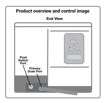
Use care to keep the hose as flat to the floor as possible. Be sure the hose is not kinked or otherwise restricted so water can pass through the hose freely. Improper installation of the drain hose may result in water leakage.
